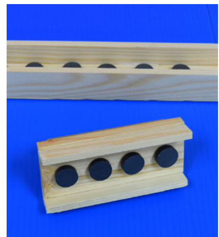
Figure 12 - Maglev train underside showing position of magnets.
