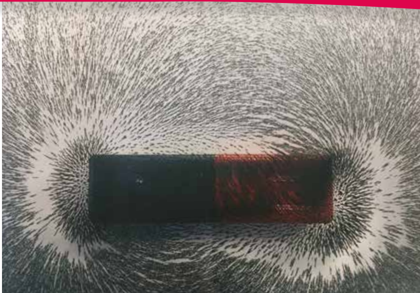
Figure 11a - Iron filings show field line around a magnet.
