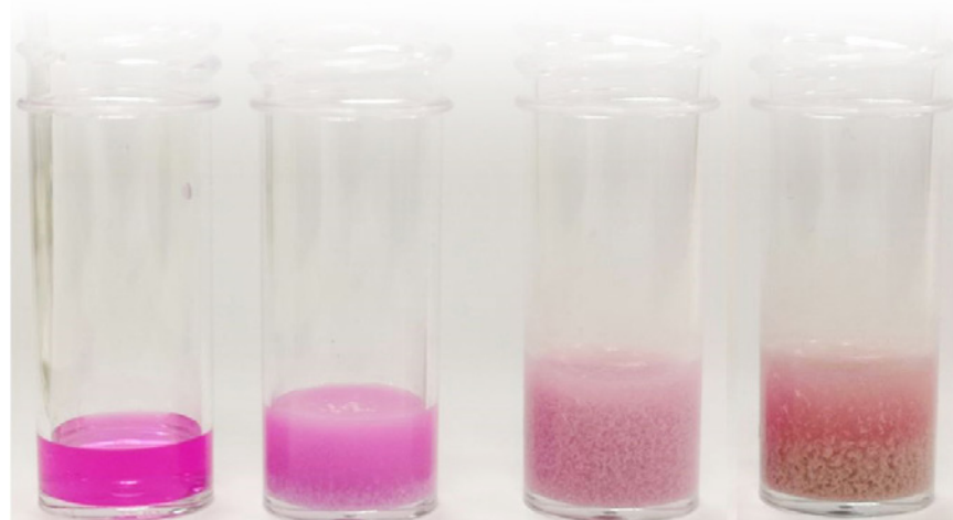
Figure 3 - Phenolphthalein. L-R Starting solution, silver chloride precipitate, end-point colour change, going further.
