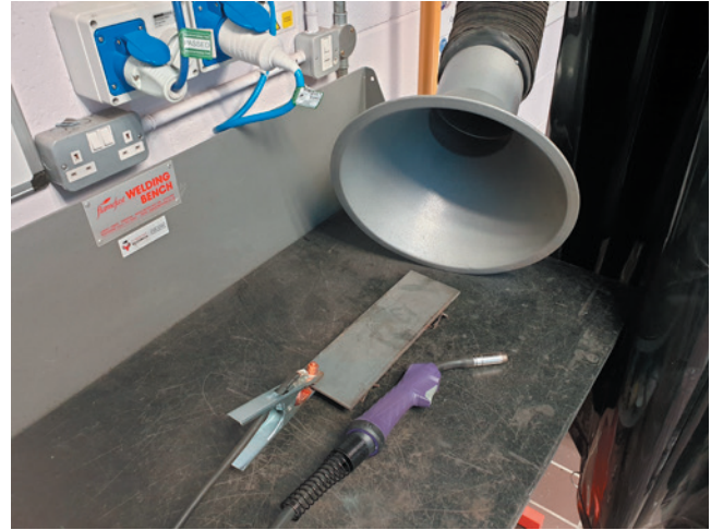
Figure 1 - Welding booth showing movable extraction arm/hood.
