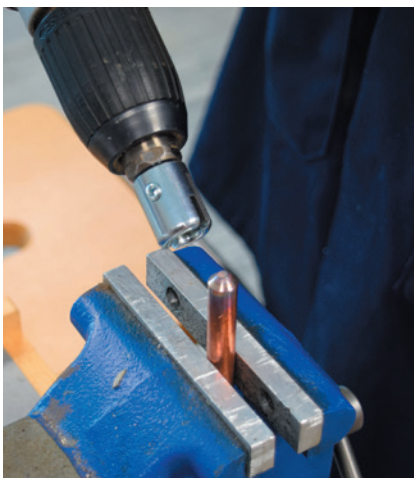
Figure 8 - Electrode cutter fixed into drill chuck.
