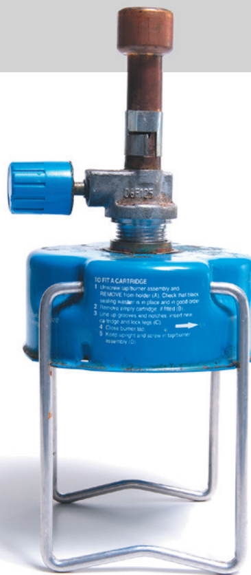
Figure 1 - Attachment for camping gas cylinder. NOT to be used in schools (image Lilly_M under Creative Commons license 3.0).
