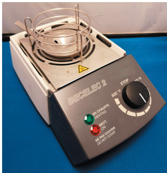
Figure 5 - An electric 'burner'.
