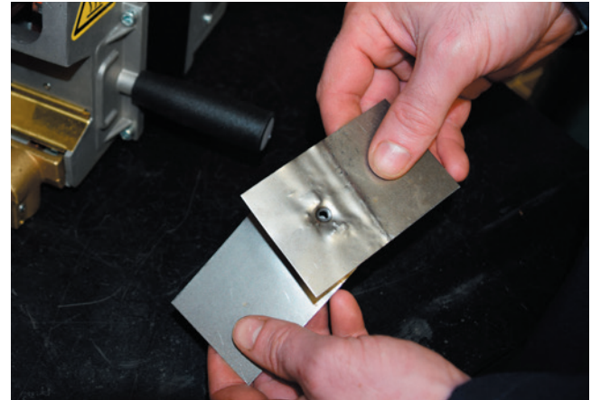
Figure 10 - Testing weld quality.
