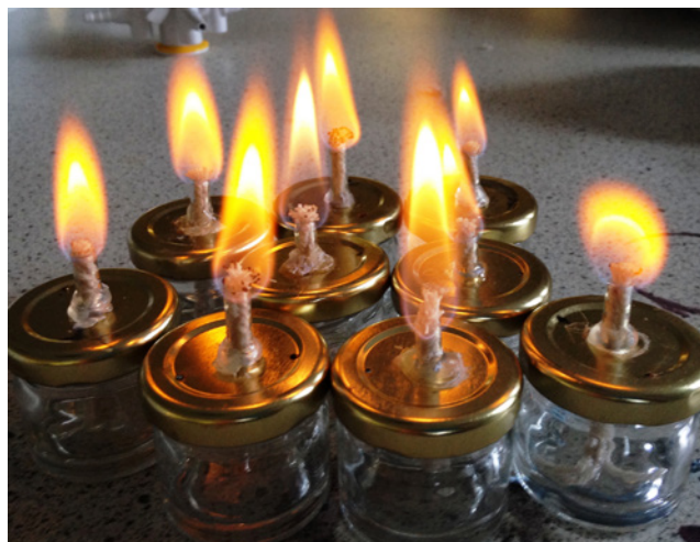
Figure 3 - Homemade spirit burners.
