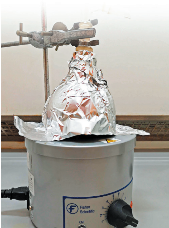
Figure 4 - A heating mantle wrapped in foil to help achieve higher temperatures.
