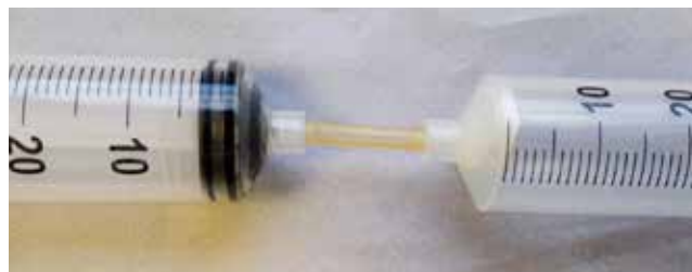
Figure 7 - Connecting two syringes using a piece of tubing.
