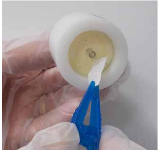
Figure 3 - Wiping an eluting source.
