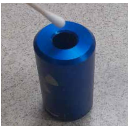
Figure 5 - Wipe the pot, not the source.
