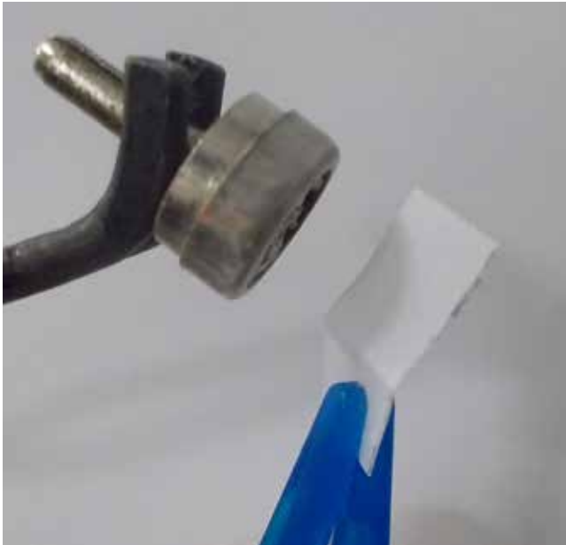
Figure 2 - Wiping the grill on a "standard" source.
