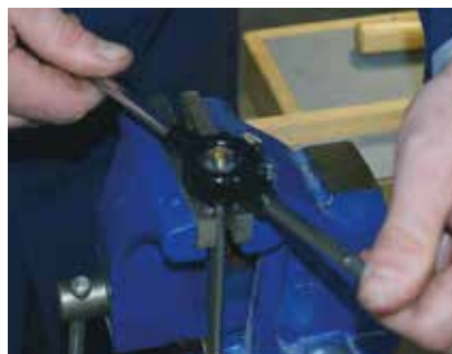
Figure 7 - Die stock turned a quarter turn back to "break" and clear the cutting.
