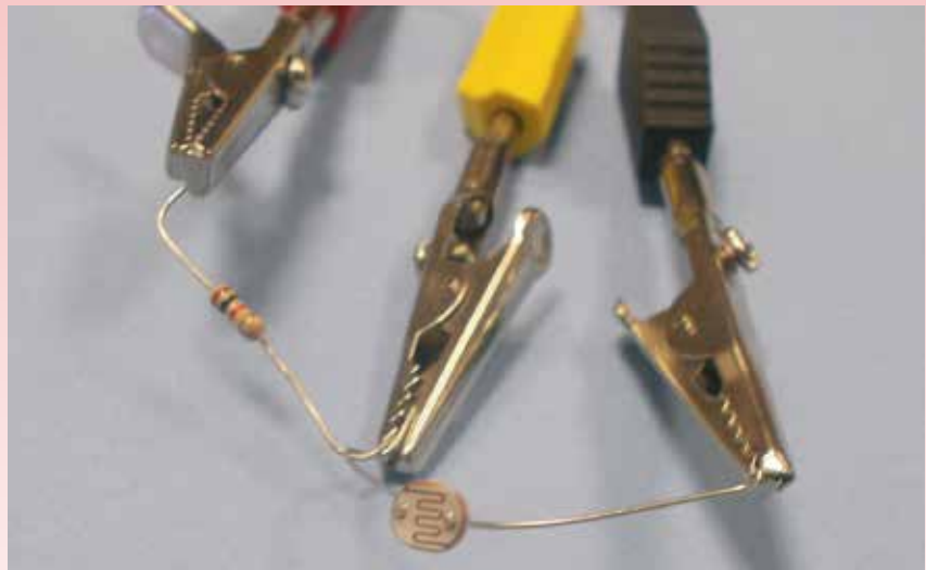
Figure 5 - LDR in potential divider.
