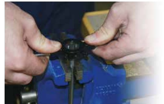
Figure 5 - Even pressure applied downwards, while being rotated. Check for square against rod.
