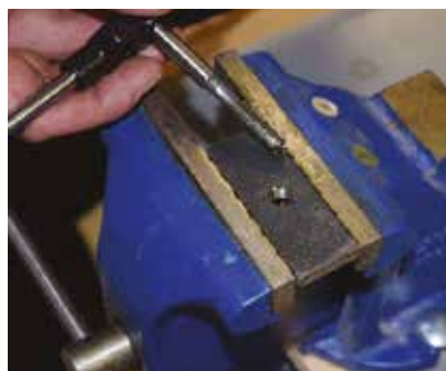
Figure 8 - Once complete, the 2 nd and plug tap should be used to fully cut the thread.
