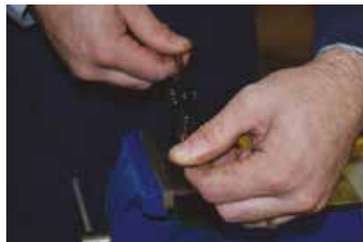
Figure 6 - Tap wrench is turned clockwise half a revolution.
