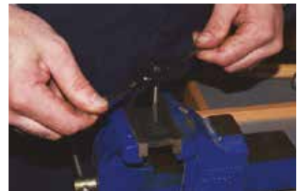
Figure 7 - Tap wrench turned back quarter of a turn to break and clear the swarf.
