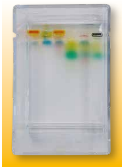
Figure 4 - An array of different colours that can be produced by electrophoresing different supermarket food colourings in agar gels using TBE buffer.
