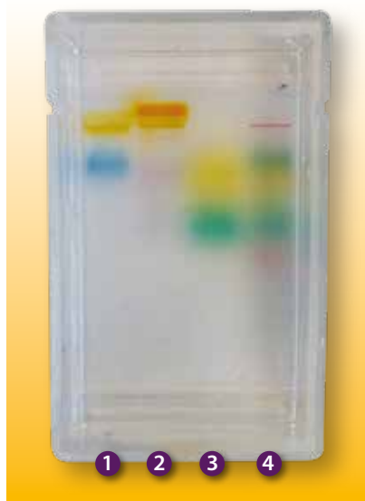
Figure 1 - 4 different green dye mixtures following electrophoresis in a 2% agar and 1 x TBE gel and buffer.
