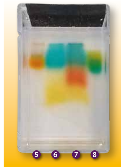
Figure 2 - 4 different green dye mixtures following electrophoresis in a 2% agar and 10 mM sodium hydrogencarbonate gel and buffer.
