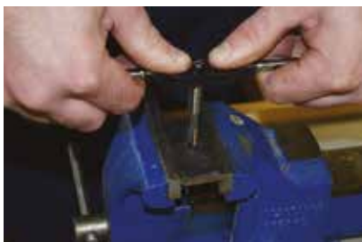
Figure 5 - Even and square pressure must be applied to initially start the cut.
