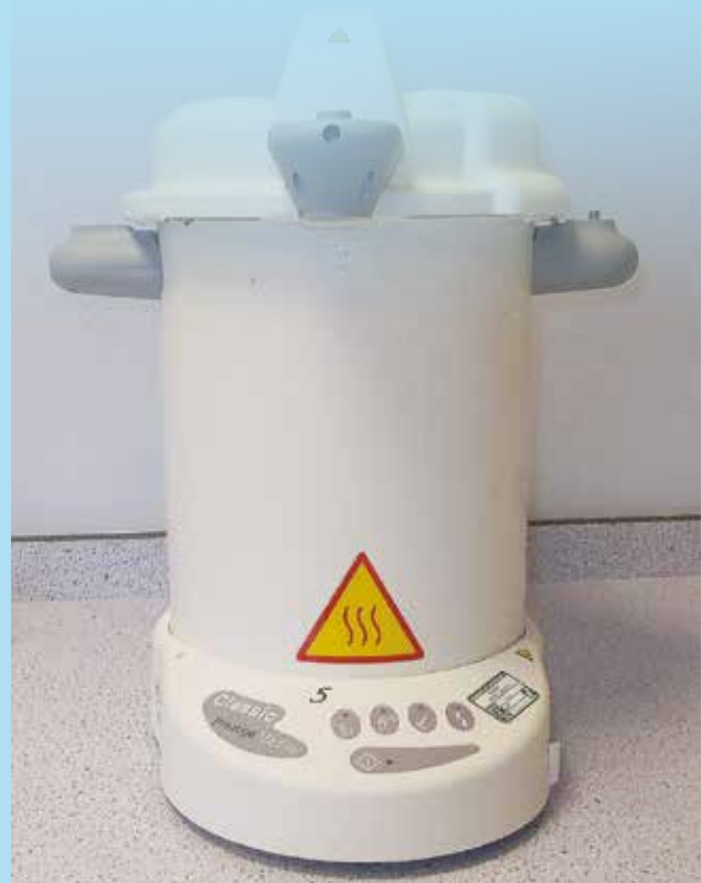
Thermostatically controlled autoclave. Note the unique identifier (numeral 5) written on it.
