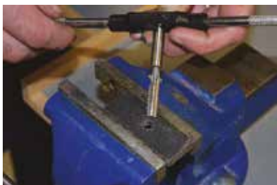
Figure 4 - To cut an internal thread the taper tap must be used first.
