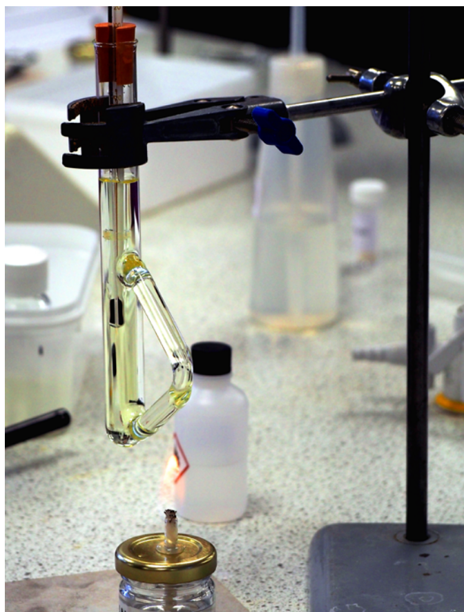
Fig 4: A Thiele tube in use
