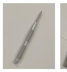
We started by turning a circular piece of aluminium. After safely securing the metal into the lathe, we faced one edge off. Then, we switched to taper turning the other edge, drilling a hole, and finishing by knurling and turning between centres. The final product was a scribe handle, and we glued the scribe piece into the section we drilled out.
