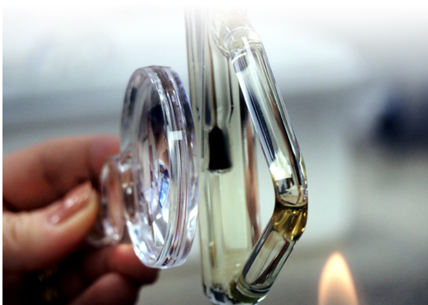
Figure 5 - Taking a reading from a Thiele tube.
