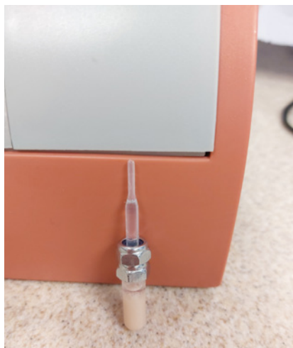
Figure 3 - A 0.2 cm 3 plastic pipette with 1 cm 3 5% yeast and 1 cm 3 10% sugar mixture held in the bulb. Two nuts are placed over the stem as weights.
