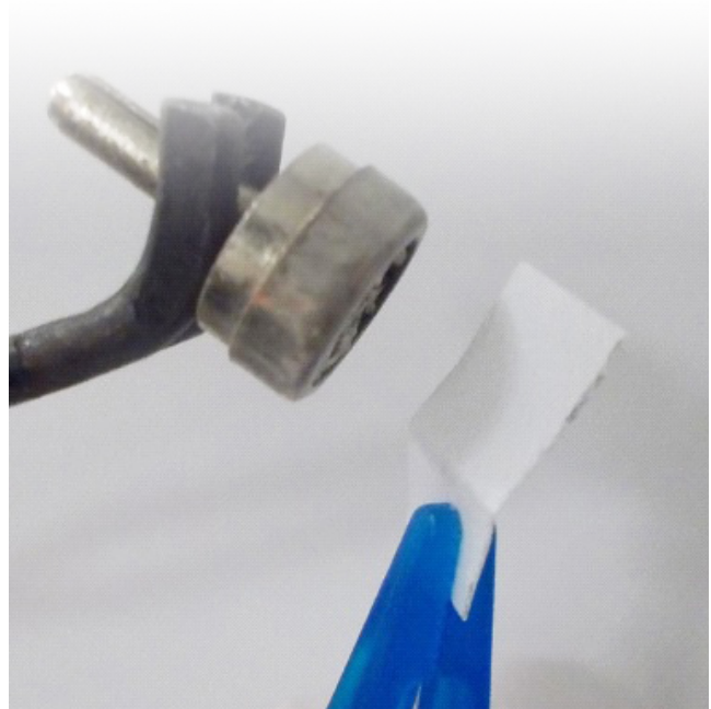
A source undergoing a leak test.
