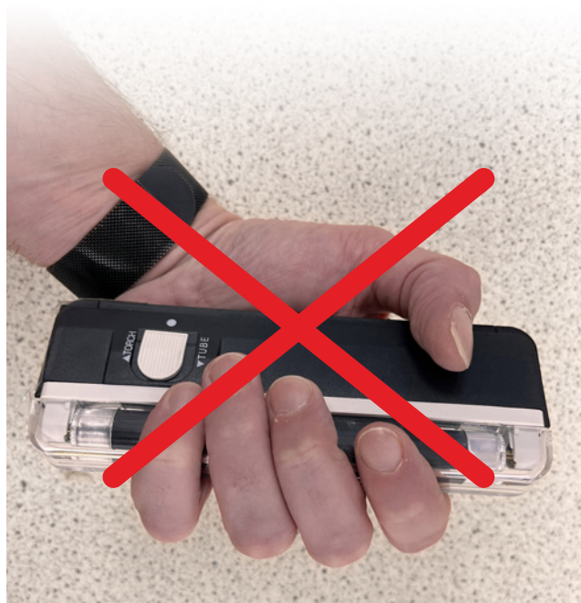
Figure 1 - Guidance states that individuals must not carry UV lamps with fingers across the tube.
