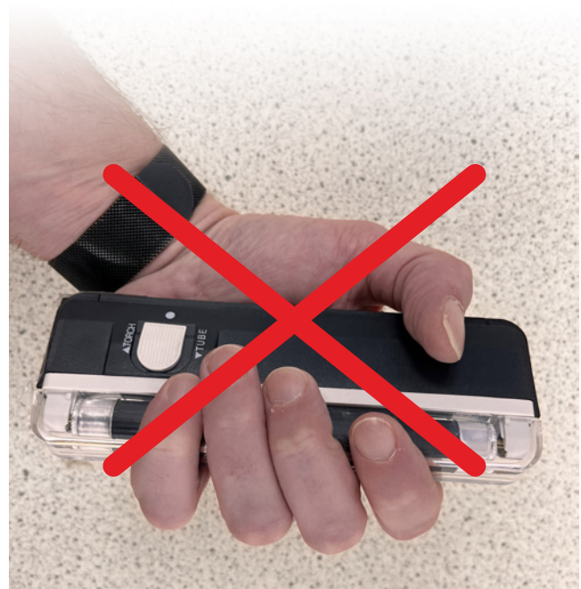
Figure 1 - Guidance states that individuals must not carry UV lamps with fingers across the tube.
