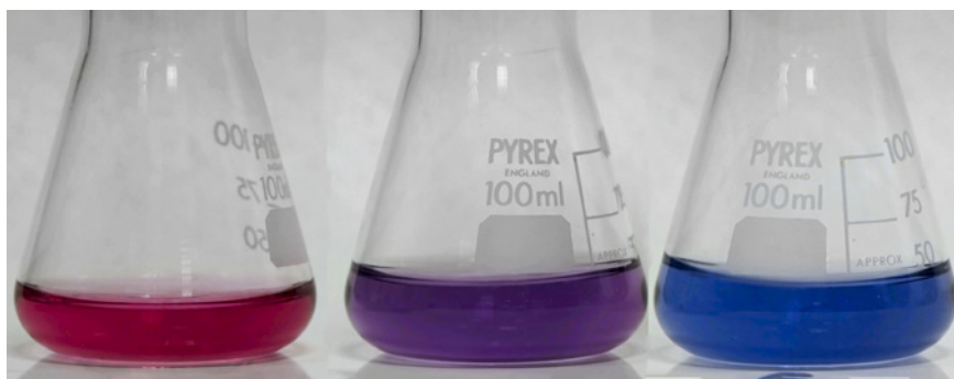
Figure 4 - Colour changes of murexide/magnesium complex (l) and uncomplexed murexide (r).
