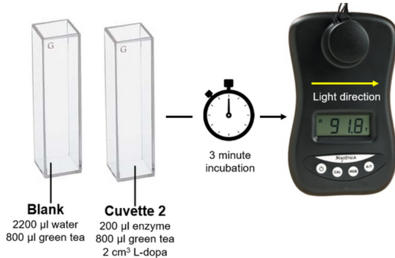
Figure 3: Integrated diagram to show assay to test the effect of green tea on dopa oxidase activity. The colorimetric blank must include the same proportion of green tea as in the test sample (cuvette 2) to account for the colour of the solution.
