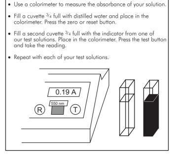
A colorimeter can be used to measure the amount of light absorbed by the coloured solution. Different colours absorb different wavelengths of light to a different extent, so we shine light of a single wavelength through the mixture. It is best to use green light (wavelength 550 nm), because the colours of the indicator (purples, reds and yellows) absorb green light quite well.
