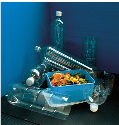
Figure 1 Basic components for a compost column cut from 2 litre drinks bottles. Also shown are some of the types of vegetable matter used to fill such a column.
