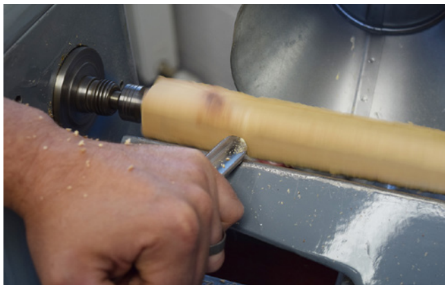
Figure 3 - Gouge tool position.
