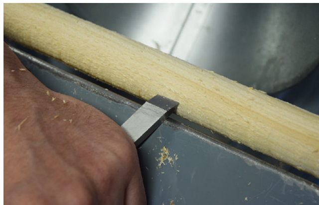
Figure 4 - Skew chisel position.
