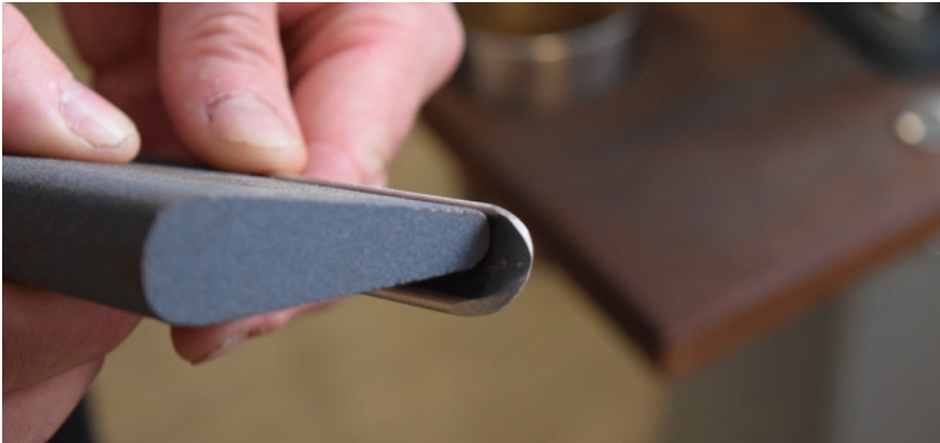
Figure 8 - Burr removed using a wet/oilstone slip.
