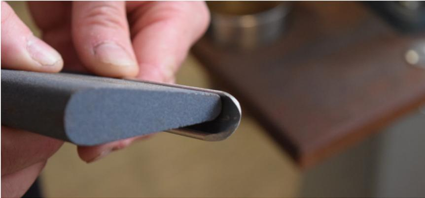
Figure 8 - Burr removed using a wet/oilstone slip.
