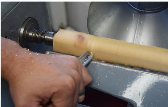
Figure 3 - Gouge tool position.
