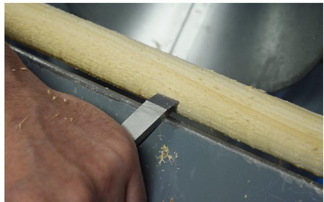
Figure 4 - Skew chisel position.
