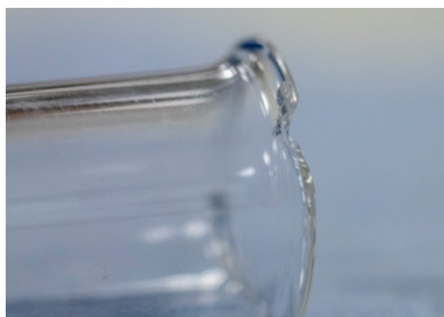
Figure 3: Chip in a test tube
