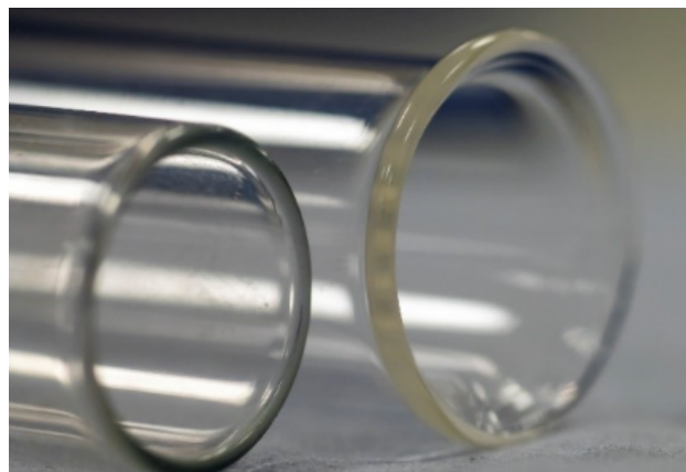
Figure 2: Test tubes with and without rim
