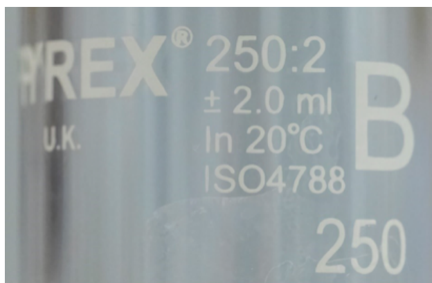
Figure 1: markings on a measuring cylinder
