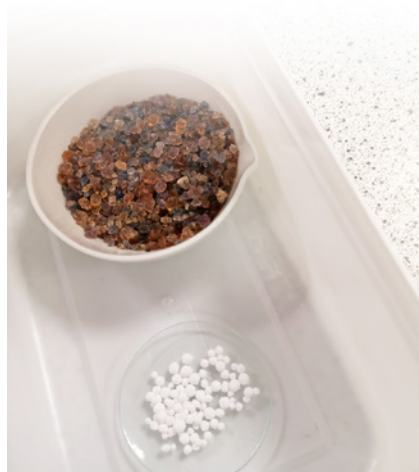
Figure 2 - A DIY desiccator.
