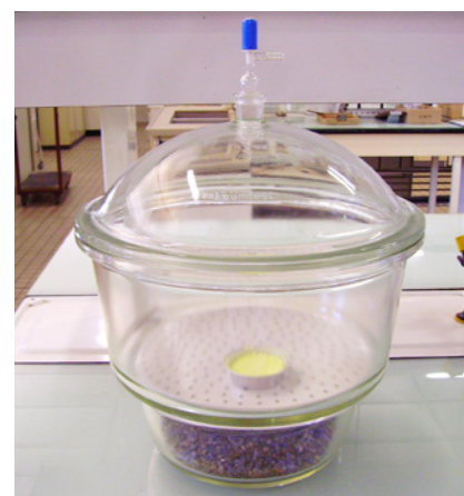
Figure 1 - A vacuum desiccator. Image by Cjp24 on Wikimedia Commons under a Creative Commons License.
