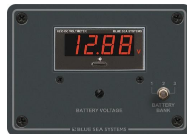
The voltage is 12.88 \pm 0.01 V
