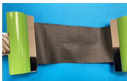
Figure 3 - The lines of equipotential are drawn out by the parallel lines of dots made by the probe making out points at the same potential.
