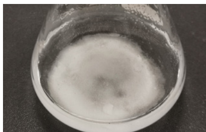
Figure 1 - If there is no water in the liquid, your drying agent will remain as fine grains – like this sodium sulphate.
