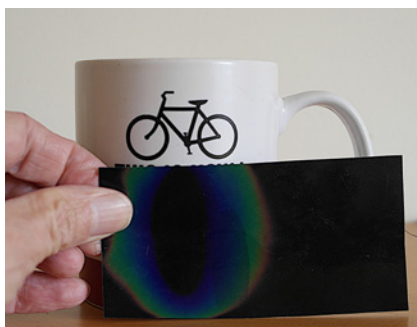
Figure 1 - Warm water in a mug causing thermochromic film to change colour.
