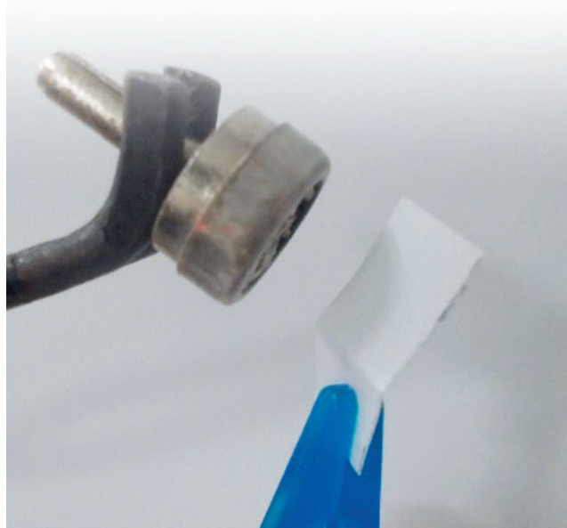
Figure 1 - A source undergoing a leak test.
