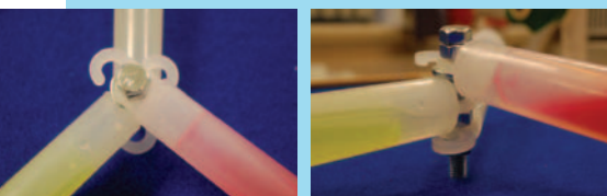
Figure 2 - Joining the light sticks together. The angle between the sticks is set to be approximately 120°.
