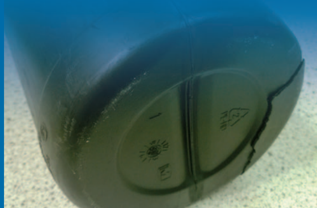
Figure 1 - A nitric acid bottle showing severe cracking.
