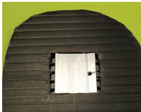
Figure 9 – Place the aluminium square in the square cut out for it in the top layer of Corriflute.
