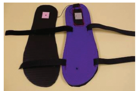
Figure 14 – Thread the Velcro through the slots cut in the flip flop.
