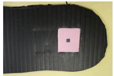
Figure 11 – Cut a 3 x 3 cm square piece of foam. Cut a 3 x 3 mm square hole in the centre of the square foam for two pellets of QTC to fit in, one on top of the other. Place the foam square on top of the aluminium square located in the Corriflute.
