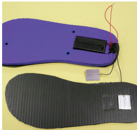
Figure 10 – Strip 1 cm from the end of the red wire attached to the battery and 1 cm from the end of the red wire attached to the buzzer, twist or solder these bare wires together to make a good electrical connection. Strip 2 cm from end of the black wire connected to the buzzer then thread it through the hole in the second 3 x 3 cm square of aluminium. Twist the wire round itself as described previously or solder to make a good electrical connection between the buzzer and the second sheet of aluminium.
