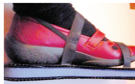
Figure 19 – Attach the shoes to your shoes using the Velcro fastening. Walk along and every time pressure is applied to the heel a buzzing sound will be heard. Remember to switch the battery off after use.
