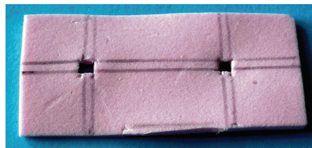
Figure 1 - Cut a 3x 6 cm piece of foam and mark on 3 x 3 mm squares for the QTC pellets 1.5 cm from each end and from each side. Using a sharp pair of scissors cut out the squares in the foam sheet. Insert one QTC pellet into each of the square holes.
