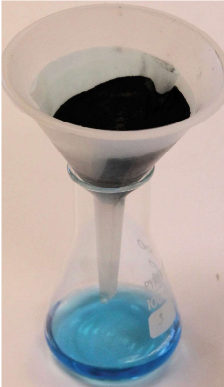
Figure 3 - Filtering and made up to 100cm 3 in conical flask.
