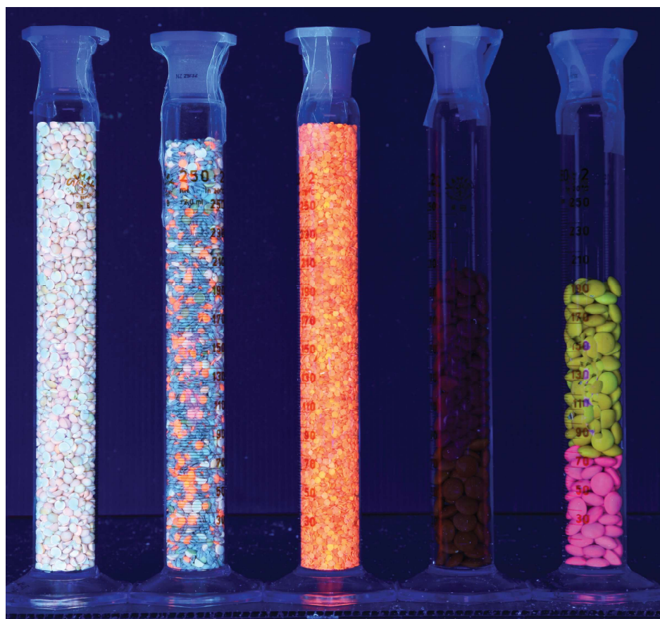
Figure 6 - The effect of UV light (365 nm) on (from left) of split yellow peas, soup and broth mix, red split lentils, red and brown Smarties®, yellow and blue Smarties®.
