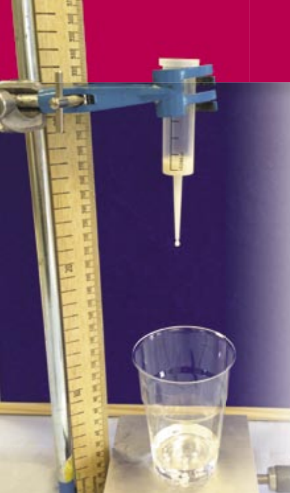
Figure 1 - Experimental set-up for producing immobilised yeast balls.
