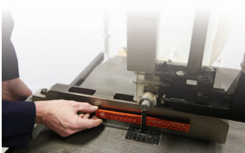
Figure 2 - Central magnets allow the Band Saw Buddy to be attached directly to the blade.
