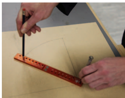
Figure 4 - Diameter/radius marking holes.
