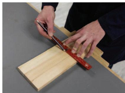
Figure 5 - Accurate straight edges for marking out.
