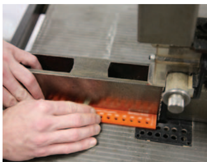
Figure 3 - A 20 mm accurate thickness gauge.
