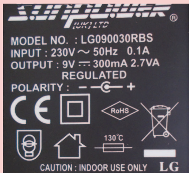
Figure 7 - Rating information on a plastic-bodied plug top PSU.
