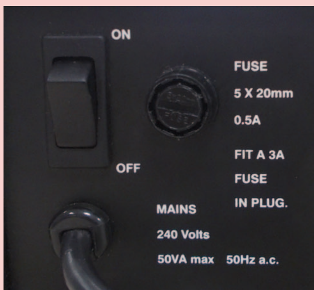
Figure 6 - Rating information on a metal-bodied PSU.
