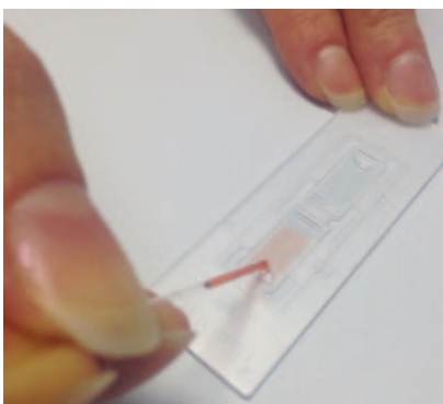
Figure 10 - Use a coloured liquid to practise loading the haemocytometer.
