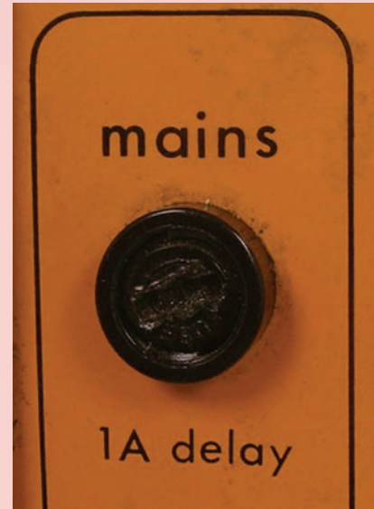
Figure 4 - Well-designed mains fuse holder.
