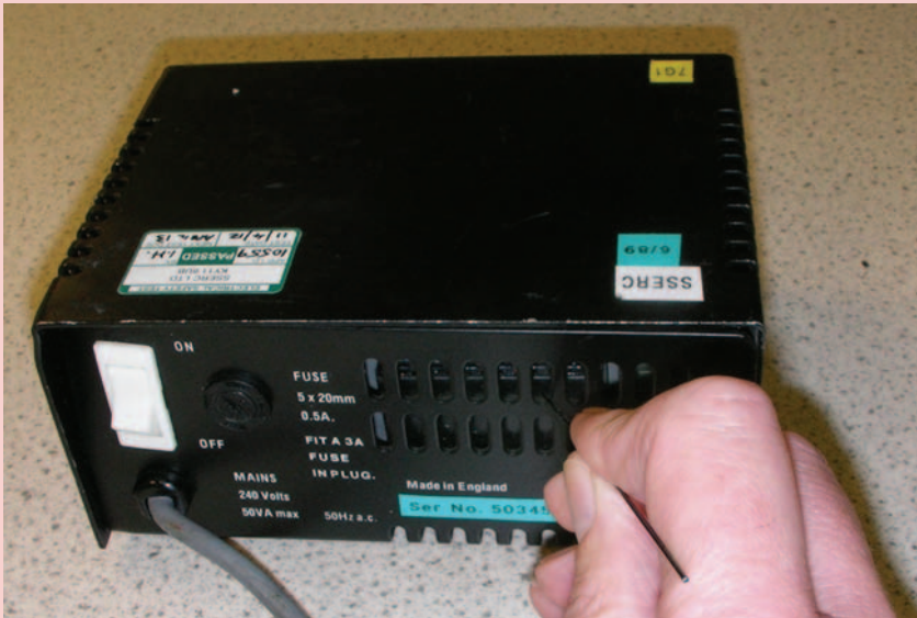
Figure 3 - Pupils might be tempted to stick things into vent holes.
