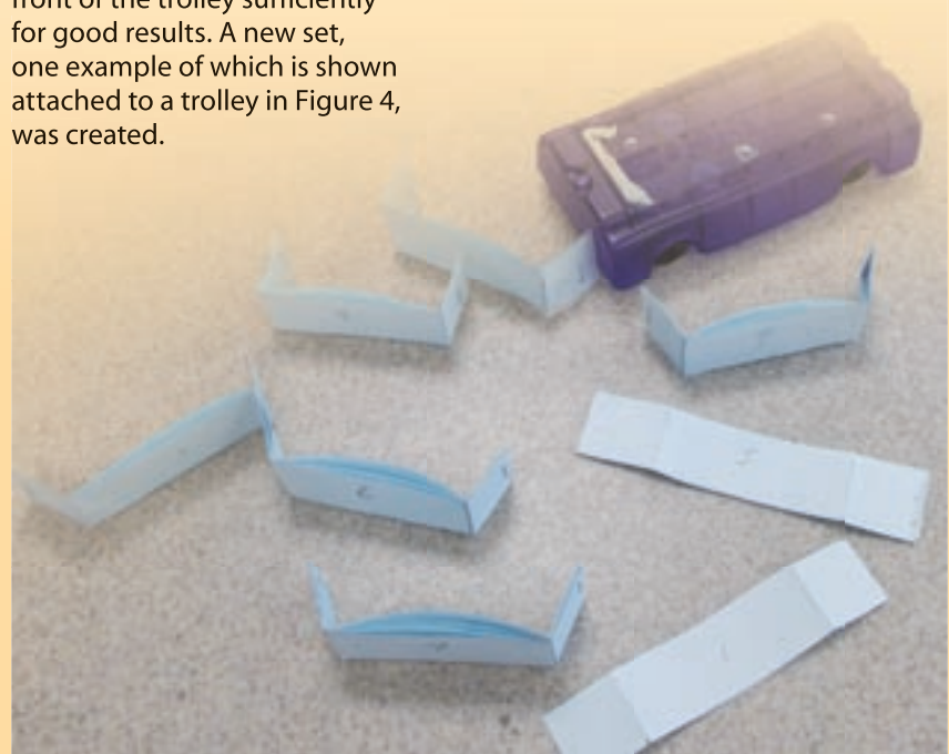
Figure 3 - Trolley with crumple zones of varying thickness.
