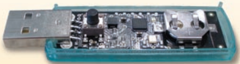
Figure 1 - USB accelerometer with lid removed to show circuitry. Because we're physicists.
