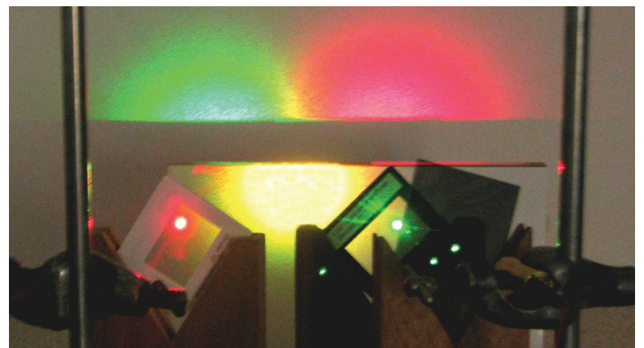
Figure 2 - Red and green mix giving yellow. The 2 LDMs are held in bossheads in the foreground. The pieces of LSD and the polarizer are in wooden lens supports.
