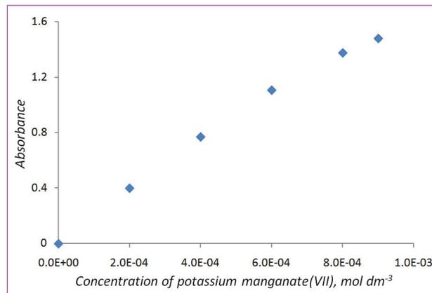
**Figure 4** - Absorbance, as measured using the Mystrica Colorimeter, as a function of the concentration of aqueous solutions of potassium manganate(VII). Excitation wavelength was 535 nm and pathlength was 1 cm.
