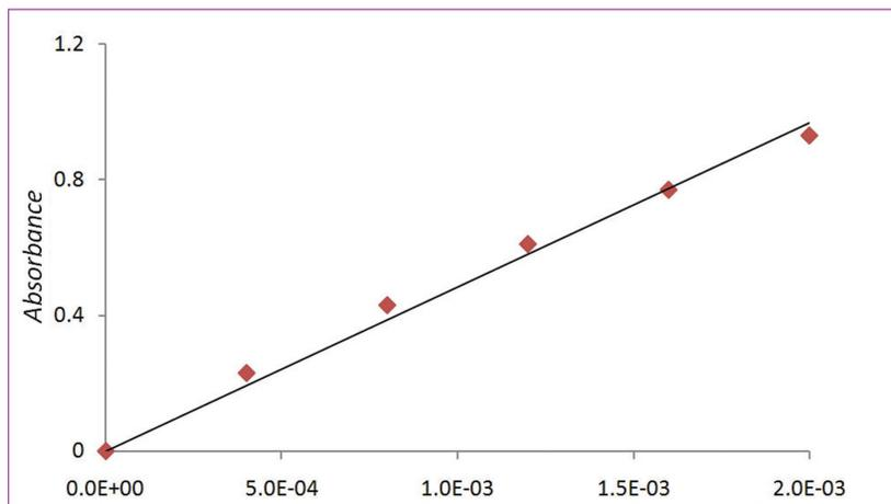
Figure 9 - Absorbance, as measured using the Mystrica Colorimeter, as a function of the concentration of aqueous solutions of methylene blue. Pathlength was 1 cm.
