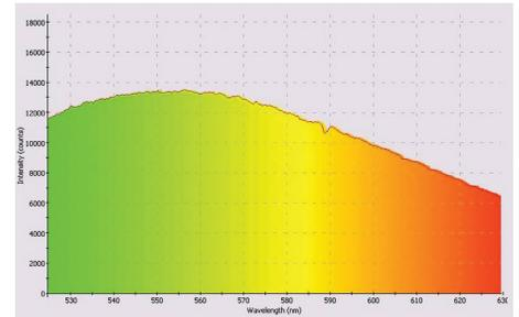
**Figure 13 - Sodium absorption spectrum. Note the wee nick in the spectrum at around 589 nm where most absorption takes place.**
