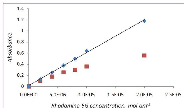
**Figure 5** - Absorbance as a function of the concentration of aqueous solutions of rhodamine 6G. Excitation was 535 nm and pathlength was 1 cm. The colorimeter used was either a CO7500 colorimeter using a 520 nm filter (♦) or the Mystrica Colorimeter (■).
