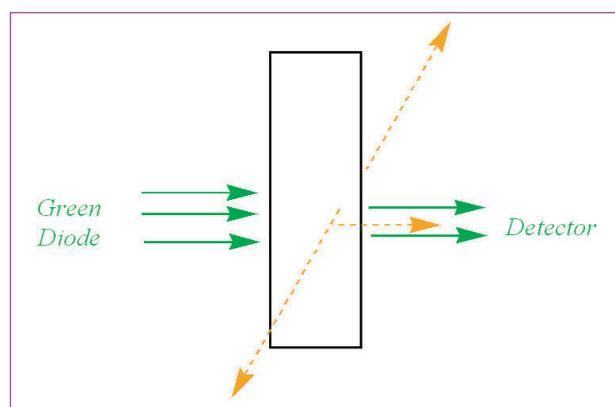
**Figure 7** - Here fluorescence is emitted in all directions and, since there are no filters in place, some of this may fall on the detector. Even though light has been absorbed in the solution the detector does not 'see' this by way of the full reduction in intensity which might be expected since some of the green light has been converted into orange light which the detector also collects. So the apparent absorbance in the cuvette is lower than the actual/true value.
