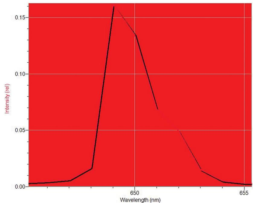
Figure 15 - Spectrum from laser diode module (Red Tide).
