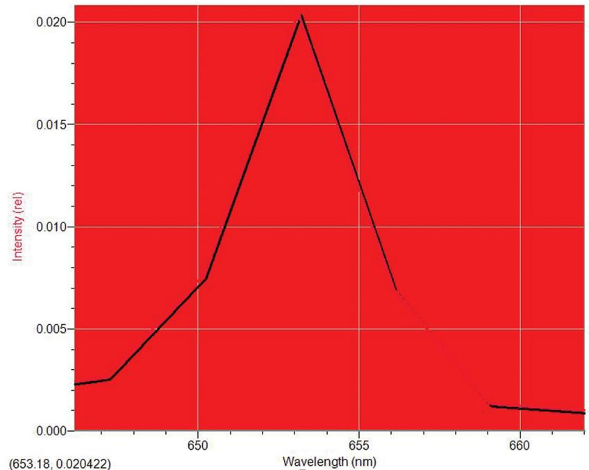
Figure 14 - Spectrum from laser diode module (SpectroVis).
