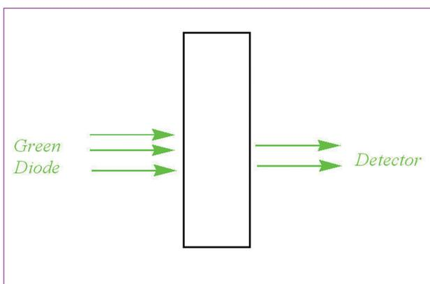
**Figure 6** - The detector collects all light. Light which is absorbed in (say) a potassium manganate(VII) solution reduces the amount falling on the detector and the change in intensity is converted into an absorbance reading.
