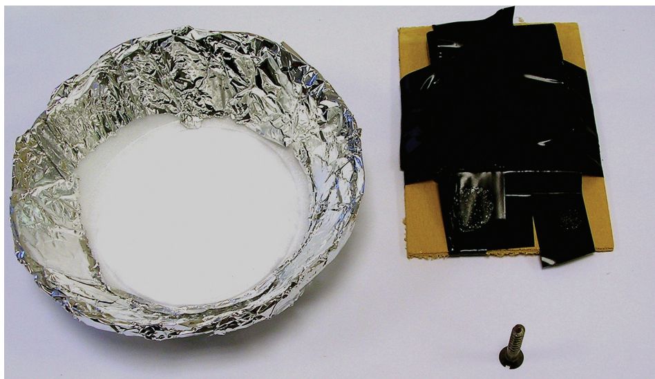
Figure 1 – Parts of a magnetohydrodynamic motor (batteries and leads not shown)
