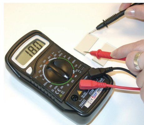
Figure 4 – The low resistance reading on the multimeter shows that this is the conducting side of the clear glass electrode. ▶
