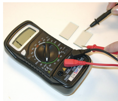
Figure 3 – The multimeter indicates that this is the non-conducting side of the clear glass electrode.
