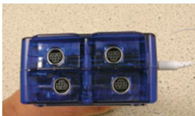
Figure 2 - Sockets for Passport sensors
