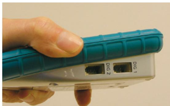
Figure 9 - Labquest digital ports
