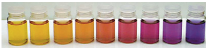
Figure 1: Effects of different concentrations of CO 2 on the colour of hydrogencarbonate indicator
