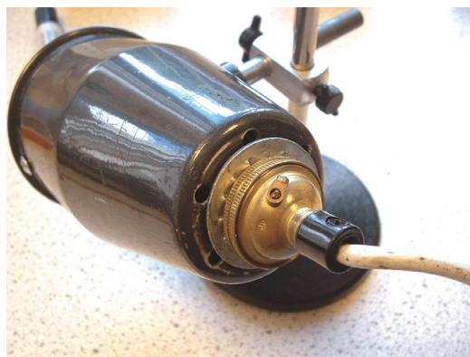
Figure 4 - Lampholder secured with shakeproof washer.
