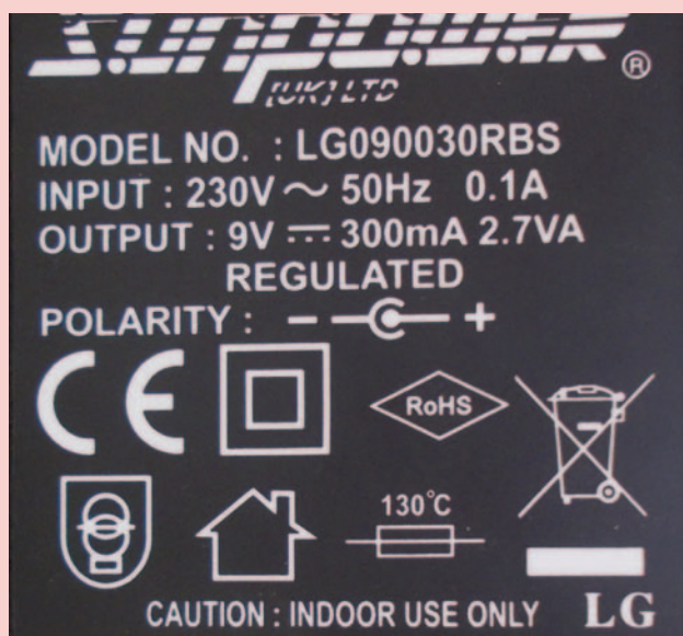
Figure 7 - Rating information on a plastic-bodied plug top PSU.
