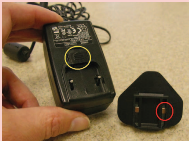
Figure 1 - Plug top with detachable blade.
