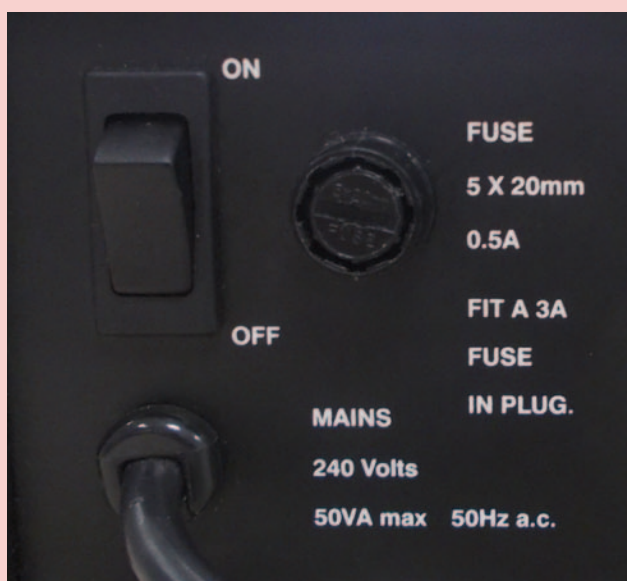
Figure 6 - Rating information on a metal-bodied PSU.
