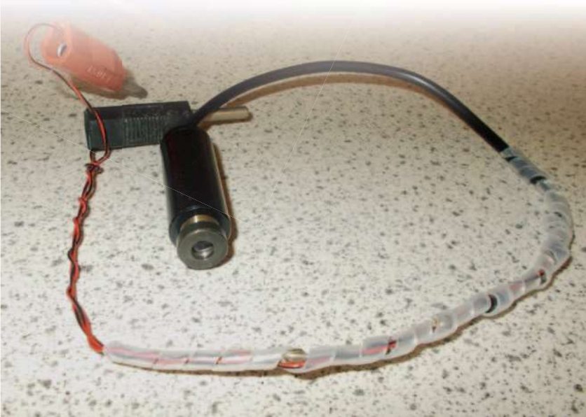
Figure 1 - The violet LDM with chain of diodes.
