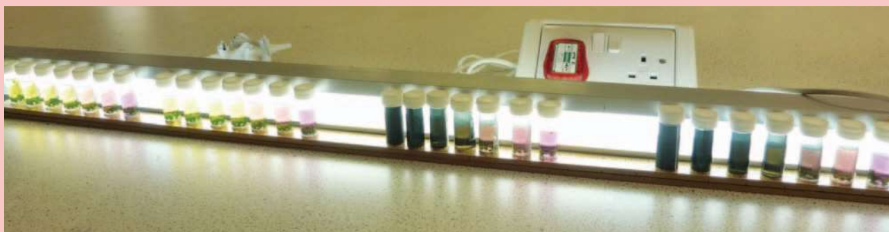
Figure 6 - An experimental set-up allowing for measurement of the effects of light intensity on the rate of photosynthesis. Bijou bottles containing immobilised algae are exposed to light from a fluorescent tube; light intensity is altered by the addition of a suitable filter.
