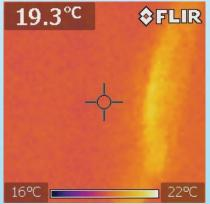
Figure 7 - Friction heating of a carpet.
