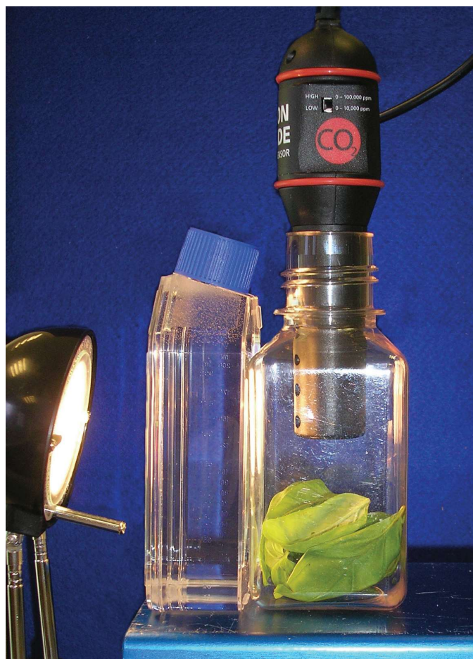
Figure 4 - Experimental set-up for measuring respiration and photosynthesis rates in plants.
