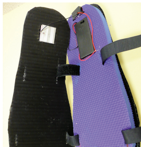
Figure 16 – Push the aluminium square sandwich into the square insert cut in the top piece of Corriflute and Sellotape it in position. Thread the Velcro through the slits in the top piece of Corriflute and pull it through so the two pieces of Corriflute and the flip flop are held firmly together.
