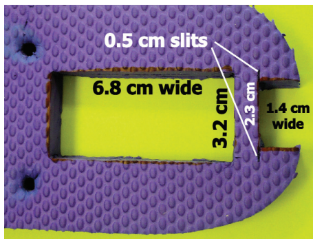
Figure 6 – At the heel end of the flip flop cut out a 2.3 x 1.4 cm shape for the buzzer to fit in. The buzzer has two mounting sockets, to accommodate these cut two slots 0.5 cm in length. The slots will hold the buzzer in place. One centimetre from the buzzer opening cut out a rectangle 6.8 x 3.2 cm for the battery holder.
