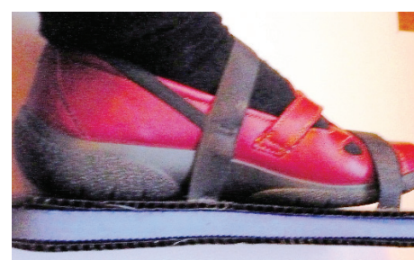
Figure 19 – Attach the shoes to your shoes using the Velcro fastening. Walk along and every time pressure is applied to the heel a buzzing sound will be heard. Remember to switch the battery off after use.
