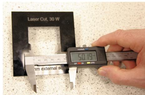
Figure 2 – Measuring the external 50 mm square.
